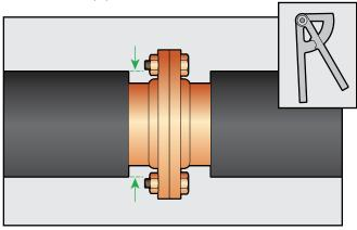
• Using caliper, measure circumference of flange.
