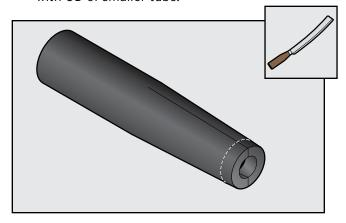
Cut end of larger ID side so length of reducer is 1/2" longer than opening to allow for 1/4" compression on each side.
