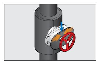
Measure circumference (C) of cover with strip of AEROFLEX Sheet the same thickness (do not stretch); add 1/4" [.64 cm] to measurement.
