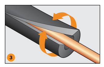
**4. Cutting:** use sharp non-serrated knives. Knife should be maintained at low angle to prevent tip from cutting/slitting inside wall. Cut flattest side of tube. Measure and cut all lengths (tube and sheet) long +1/8" [.32 cm] on each side (1/4", .64 cm) to install under compression. Use sharpened pipe cut-offs for holes. Glued seams should never be stretched and under stress.
