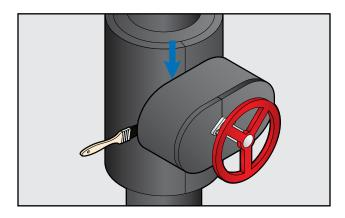
Glue edges of spindle housing jacket to face plate cover with AEROFLEX adhesive under compression.
