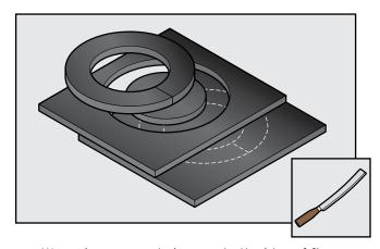
Wrap rings around pipes on both sides of flange and fully adhere to insulation inserts and bolts with AEROFLEX adhesive; do not glue rings to installed pipe insulation yet.
