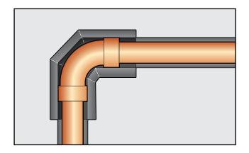
4-Piece Elbows - Welded (fitting & piping same diameter)
