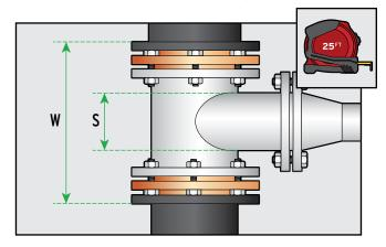
On AEROFLEX Sheet, mark and cut width (W), ring circumference (C) and diameter of spindle (S); mark spindle cut-out 1/8"-1/4" [.32 cm -.64 cm] short for compression fit.
