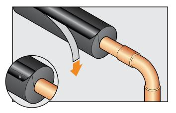
Carefully press Protape double closure seal onto clean outside wall of tube with firm pressure, avoiding any kinks or gaps, until the Self Seal tube is fully sealed.
