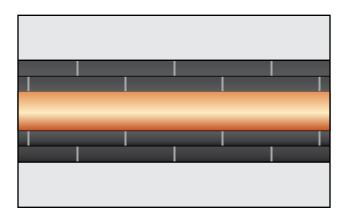
First layer of AEROFLEX sheets to be installed with full AEROFLEX adhesive coverage or AEROFLEX with PSA (pressure-sensitive adhesive back).
