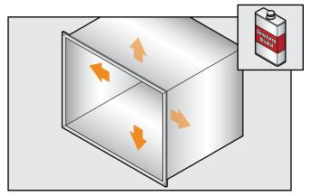
Measure duct dimensions and cut AEROFLEX Sheet & Roll with PSA with straight edge.
