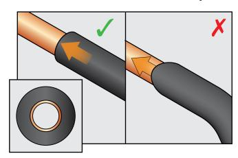
Install AeroFit or field-fabricated mitered fittings at pipe bends to prevent insulation compression (reduced thickness) and condensation.
