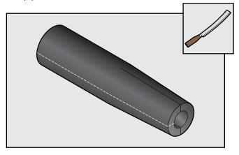
Glue reducer seam and butt joints under compression with AEROFLEX adhesive.
