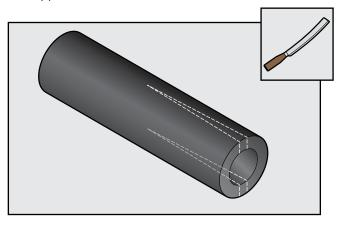
Glue notched edges together with AEROFLEX adhesive
