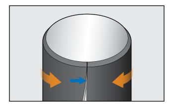
Measure the diameter of the dome using a strip of AEROFLEX Sheet insulation of same thickness.
