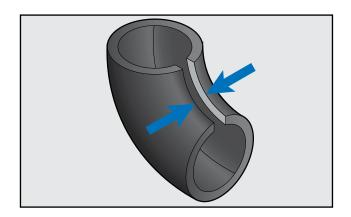
Once glued inside seam is ready for contact, wrap the fitting cover around pipe bend and apply firm pressure to ensure complete adhesion.
