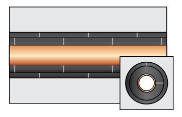
Glue butt joints under compression with AEROFLEX adhesive.
