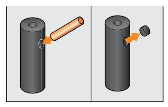
Cut main vertical tube lengthwise where it intersects with branch pipe and glue seam with AEROFLEX adhesive.
