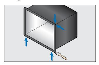
Glue four (4) flange cover edges to duct wrap with Aeroseal or Aeroseal LVOC Black under compression to create vapor seal.
