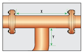
With strip of AEROFLEX Sheet the same thickness as insulation to be installed, measure the circumference of main and branch pipes (do not stretch); add 1/4" [.64 cm] to measurement.
