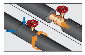
Glue valve stem, seam between valve stem, end of tube and butt joint under compression with AEROFLEX adhesive.
