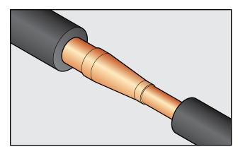
With piece of AEROFLEX tube the same ID as larger pipe, cut a section larger than opening between straight run tubes installed on either side of pipe transition.
