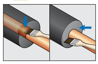
Glue longitudinal seams, butt joints and fittings with AEROFLEX adhesive. BEST PRACTICES/AEROFLEX ADHESIVES
