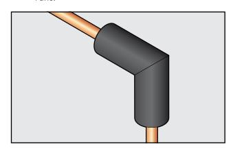
• **Note**: If straight runs are installed prior to 90° fitting cover, measure and cut fitting cover to fit with compression.
