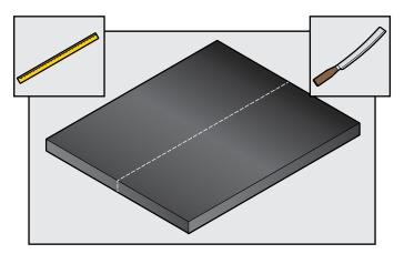
Apply AEROFLEX adhesive to cut edges of longitudinal seam, allow to tack up until ready for contact.
