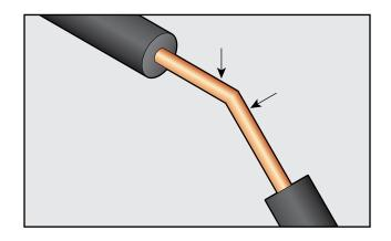
Cut AEROFLEX unslit tube at 22.5° angle using AEROFLEX Template and long sharp knife.
