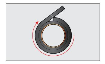
Mark and cut length of AEROFLEX Sheet & Roll with straight edge; add 1/4" [.64 cm] to measurement.
