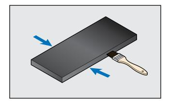
Place insulation over pipe and adhere glued longitudinal seam by pressing from the outside edges towards the middle to ensure straight edges at butt joints, full adhesion and vapor seal.
