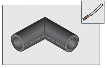
Install over pipe fitting and glue throat under compression with AEROFLEX adhesive.
