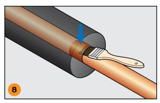
9. Taping Seams: applying zero-perm Protape over sealed seams for interior applications is recommended as an additional level of protection to prevent CUI. For pipe sizes over 6" IPS [15 cm] and sheets/rolls over 1" thick [2.5 cm], apply 2" [5 cm] Protape evenly over seams followed by 2" on either side of taped seam (4" [10 cm] total taped seam width). Protape may be applied immediately over glued seams if Aeroseal or Aeroseal LVOC Black adhesive
