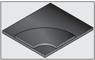
Position both sides together with smooth skin facing out and apply AEROFLEX adhesive to outer edges.
