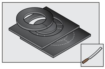
Wrap rings around pipes on both sides of flange and fully adhere to insulation inserts and bolts at flange and insulated pipes.
