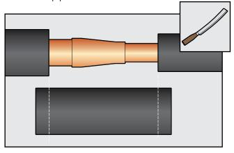
• At one end, cut two equal notches out of opposite sides to fit smaller tube.
