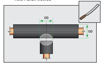
Punch hole in tube to insulate main (horizontal) pipe with sharpened pipe end of right diameter; use divider to cut hole for larger pipes.
