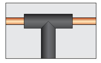
Using AEROFLEX Template, cut two 45° angles to center at end of tube for branch (vertical) pipe.
