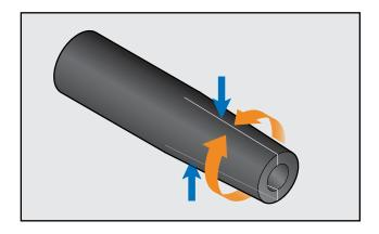
• Cut end of notched size so diameter lines up with OD of smaller tube.
