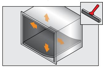
• Ensure that all four (4) inside corner edge seams fit under compression with no gaps present since it is impractical to seal them with adhesive.
