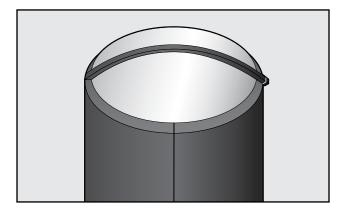
Transfer diameter measurement to AEROFLEX Sheet, draw radius and then circumference.
