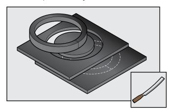
Wrap rings around pipes on both sides of flange and fully adhere to insulation inserts and bolts at flange and insulated pipes with AEROFLEX adhesive.
