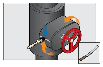
Glue edges of spindle housing jacket to valve cover body with AEROFLEX adhesive under compression.
